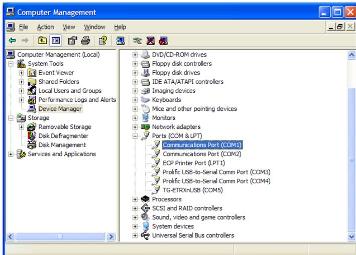
Under “Ports” you will see your Telegesis USB device(s); note the COM port number that it is attached to (here, COM5). Now you can close the Device Manager. Each board that you plug in will appear as a different COM port.
