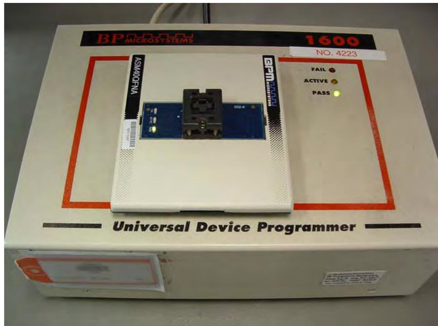
Figure 7. BP Microsystems Single-Site Manual Programmer
