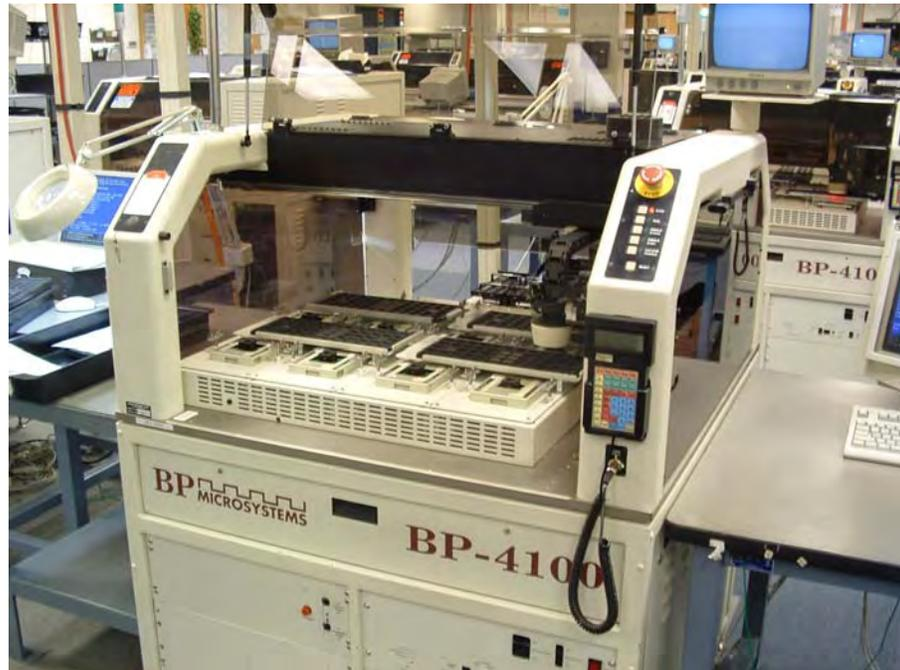
Figure 6. BP Microsystems Multi-Site Automated Programmer
