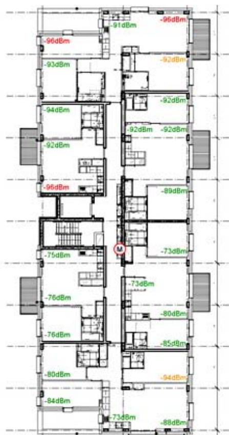
Figure 3: EDF Energy propagation tests (Source: SMDG HAN Work Group <https://sites.google.com/site/smdghanwg/home/real-world-experiences/EDF2010ZigBeePropagationTesting.pdf?attredirects=0&d=1>)
